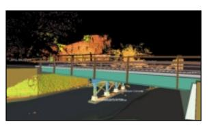
The view of scan #3 is shown after partial modeling was completed using Cyra Software.
