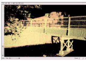
Point cloud view from scan #3. Under the foliage the bistorical stone embankment is clearly visible from this angle.
