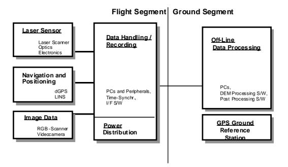
Figure 1: TopoSys system components.
