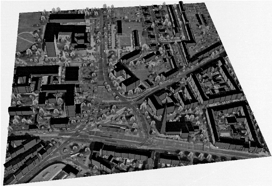
Fig. 6. 3D visualization of virtual trees and reconstructed buildings.
