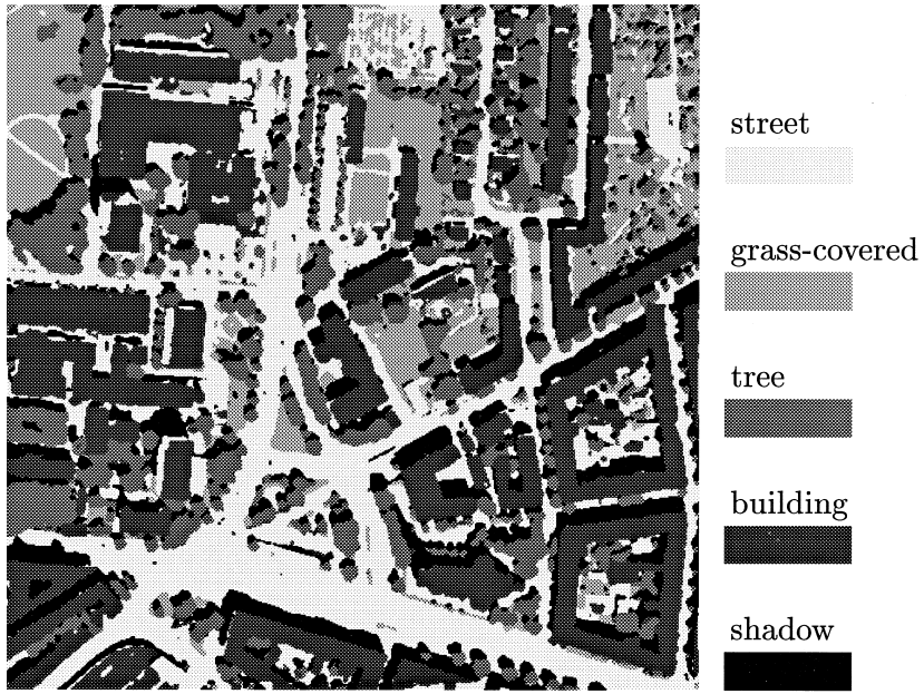
Fig. 3. Result of ISODATA classification using CIR orthoimage and normalized DSM.
