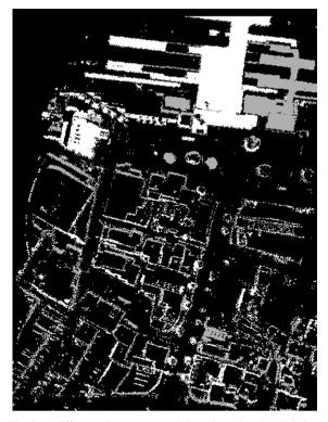
Fig. 3. A difference image generated by subtracting the ALS data acquired on October 21, 1996 from the one acquired on August 19, 1998. The white areas of the figure indicate that their elevation has become higher since the acquisition of the older data, while the grey areas indicate that their elevation has become lower than before.
