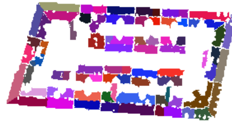
Figure 6b. Planar patches obtained by iteratively applying region growing.
